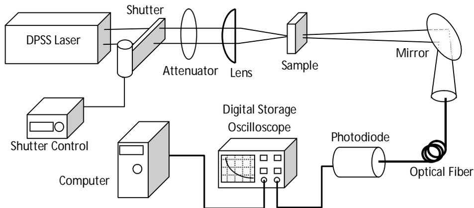
*Figure 1. Single beam transient thermal lens setup*
