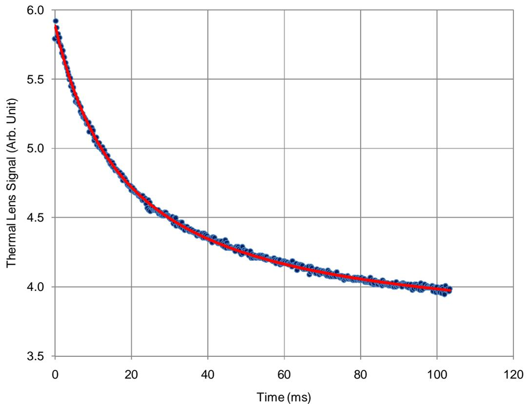
Figure 2. Typical transient thermal lens signal from Valvoline Super Kool (1:6 dilution) sample and theoretical fit to the data.
