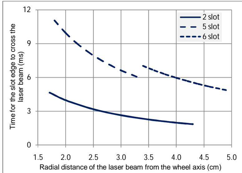
**Figure 2.** Time taken by the chopper slot edge to cross a 1mm diameter laser beam ( $1/e^2$  diameter) for different radial positions of the 2-slot and 5/6-slot wheels when operated at 4Hz.
