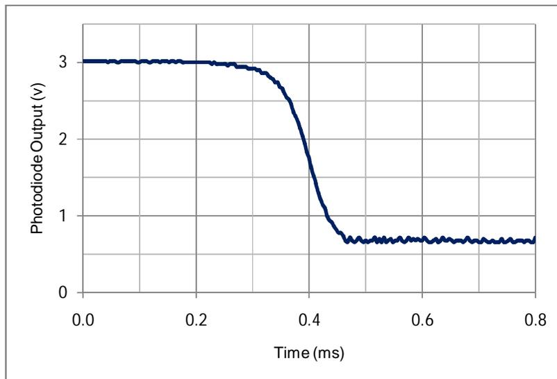
**Figure 5.** Shows the switching speed of the assembled electromechanical shutter using a 9V relay.
