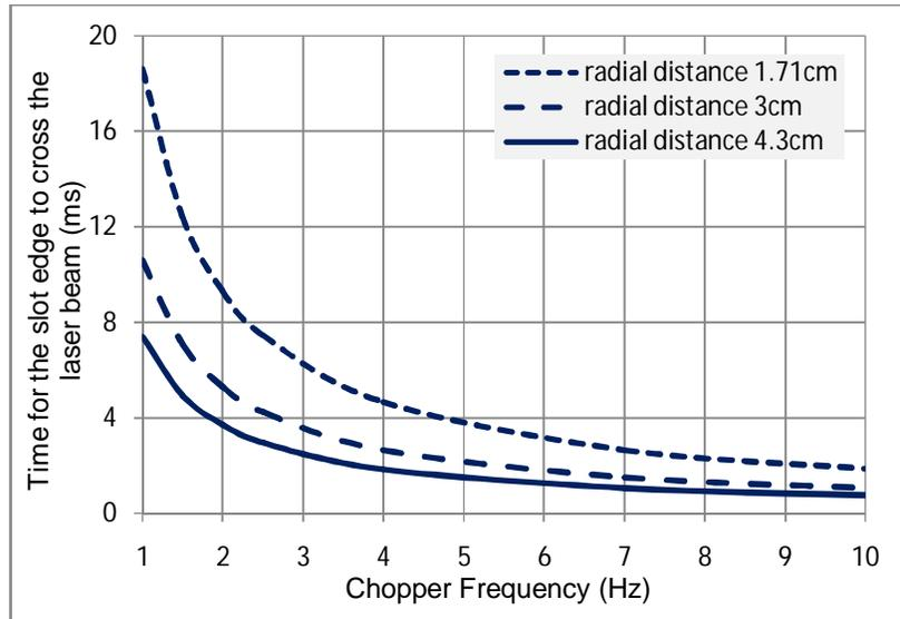
**Figure 3.** Time taken by the chopper slot edge to cross a 1mm diameter laser beam ( $1/e^2$  diameter) for different chopper frequencies by the 2-slot wheel. The three different lines show minimum, medium and maximum radial positions of the laser beam on the chopper wheel.
