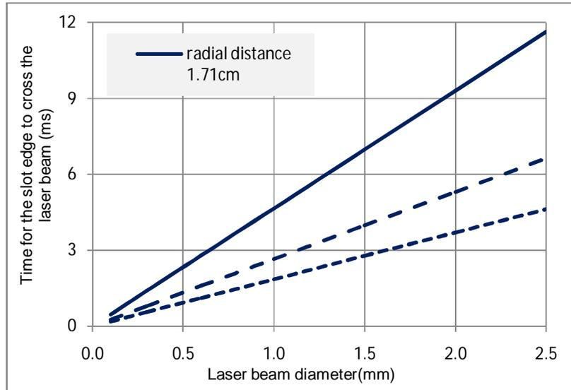
**Figure 4.** Variation of the time taken by the 2-slot wheel edge to cross the laser beam as a function of laser beam diameter. The three different lines show minimum, medium and maximum radial positions of the laser beam on the chopper wheel. Laser beam diameter of 0.1mm corresponds to a tightly focused laser and 2.5 mm corresponds to an expanded/diverging laser beam.
